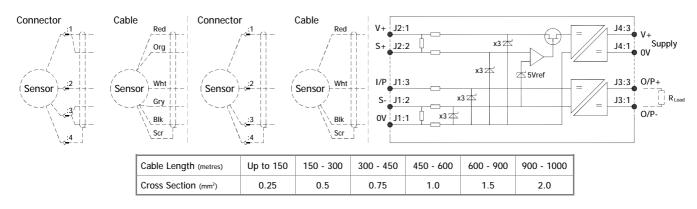
To ensure correct operation of both Amplifier and sensor, the following restrictions on conductor cross section and cable length limits are set out in the table above (figures are based on copper conductors);
