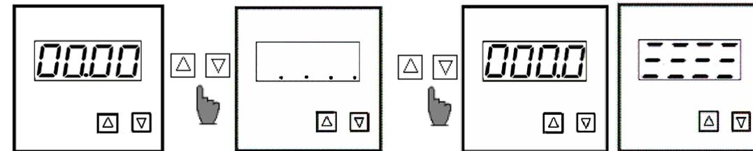
1. **Press UP/DOWN** button at the same time and continuously, until the second screen appears.
